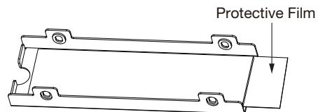
2. Remove the protective film from the thermal pad on the heatsink baseplate exposing adhesive surface. Do not remove the thermal pad itself.
