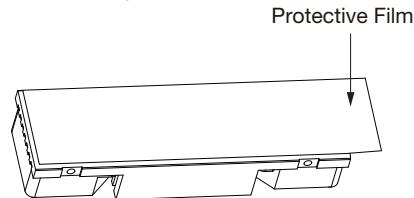
4. Remove the protective film from the thermal pad on the heatsink. Do not remove thermal pad itself. Align the heatsink's screw holes with the base plate.
