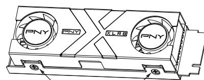
6. Fasten the heatsink to the heatsink base plate with the 4x screws from Step 1 using a Phillips #1 screwdriver.
