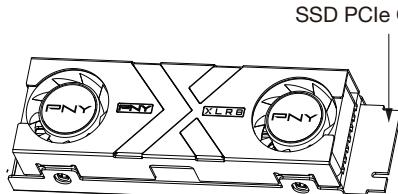
5. When placing the heatsink on top of the SSD, ensure that the fan cable is on the same side as the PCIe connector notch of the SSD. Then align the heatsink's screw holes with the base plate. Press the heatsink down until the screw holes are in alignment using even, gentle pressure.
